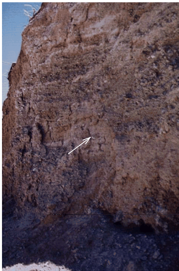
Figure 6. Example of Santa Fe Formation, showing poorly-sorted bedding and flat-lying beds. Outcrop is about 30 feet above fault clay in the detachment fault in the West Ore Zone. A six-inch scale lies at the tip of the arrow.
