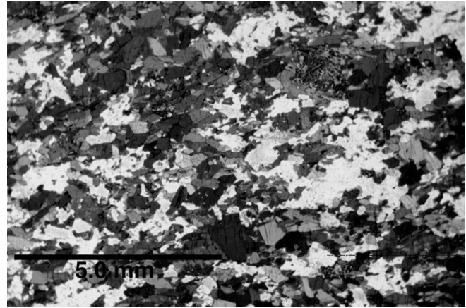
Figure 34. Amphibolitic dike rock with relict igneous texture. The original igneous mineral assemblage has been replaced by the amphibolite-facies assemblage: hornblende (gray)-plagioclase ( \sim\text{An}_{55} , colorless)-scapolite (colorless)-quartz (colorless)-sphene (colorless, high relief); however, a relict, original igneous texture is still preserved. Metamorphism was not accompanied by significant deformation in this sample. Plagioclase grains generally retain their igneous tabular habit, although they exhibit irregular grain boundaries with hornblende suggesting partial replacement, and are also partially replaced by scapolite. Unusual clusters of sphene grains in the upper right corner suggest near complete replacement of ilmenite lamellae from an exsolved titanomagnetite grain.
