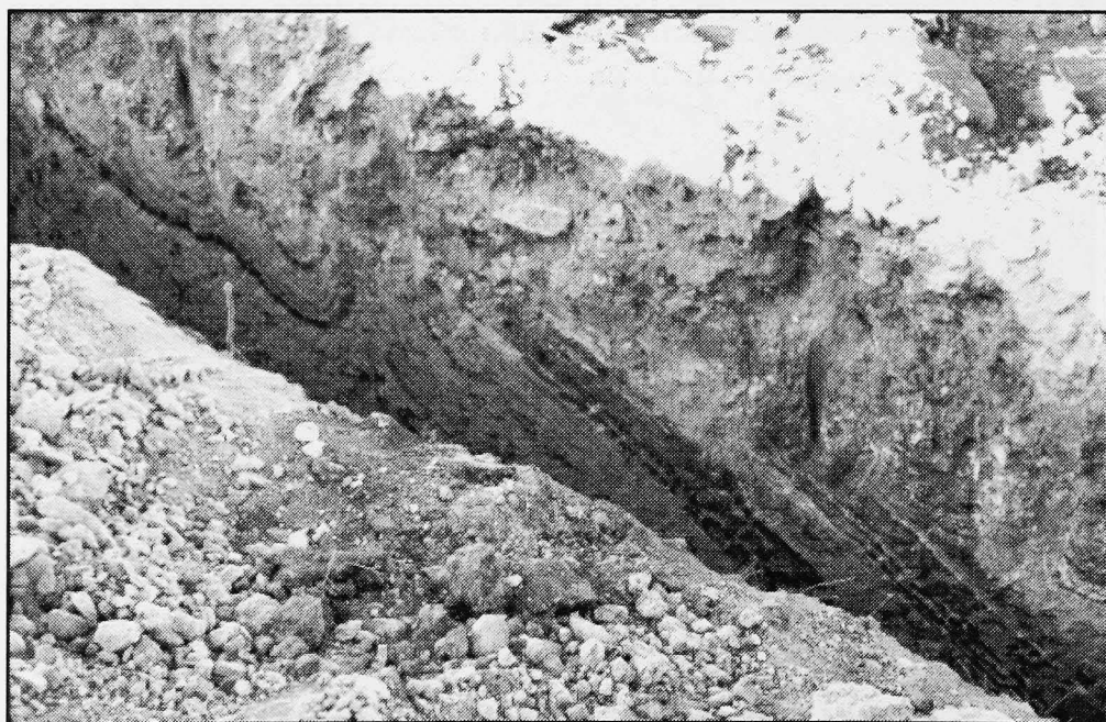
Figure 13. Smoky Hill Shale exposed in a trench in Jefferson County. Bentonite beds are seen in the trench as dark bands that are contorted on the left and steeply dipping on the right.
