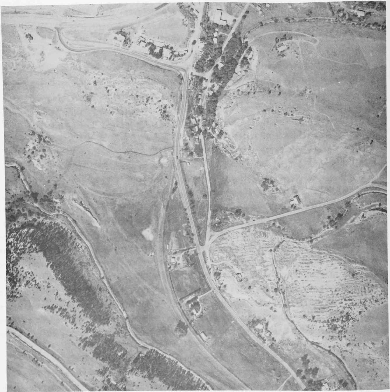
Figure 3. Local subsidence over mines in the Marshall area. The air photos were taken in 1980; figure A is a high sun angle mid-day panorama. The bottom two photos show areas in greater detail and were taken in early morning at low sun angle. The subsidence features, in shadow on the photo, correspond precisely to the rooms of the Lewis Mine as shown on the available mine maps.
