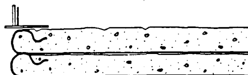
FIGURE 6 General Geotextile Wall Construction Procedure.
