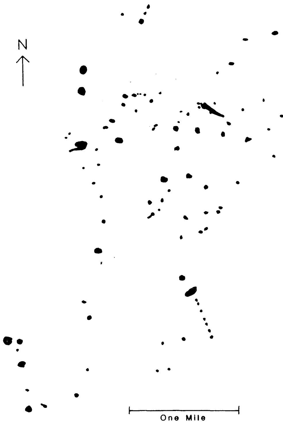
FIG.4 Distribution of sinkholes based upon existing aerial photography.
