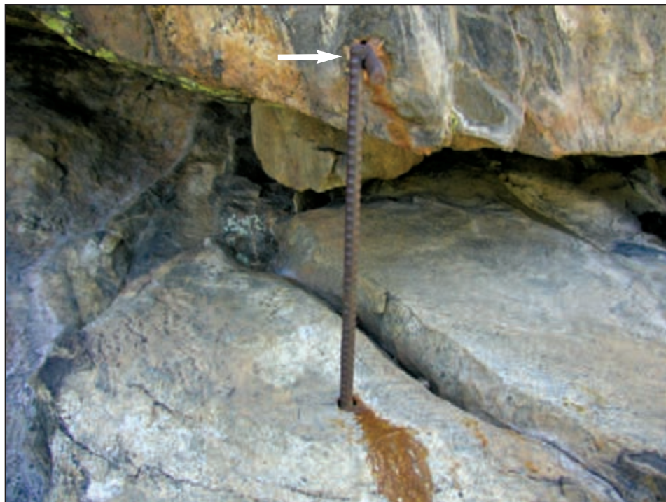
Figure 7: Close up view of tell-tale gauge. Two steel rebar segments (shown with arrow) have been cemented into small drill holes above and below the large crack in the rock. Any movement could be measured by the offset of the two bars that were touching when cemented. This rock has not moved since the gauge was installed in 2003. (Photo by Ty Ortiz, CDOT.)
