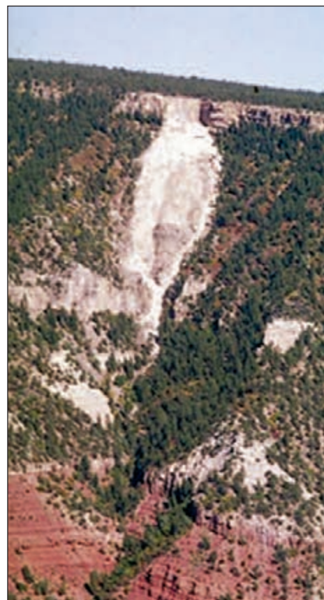
Figure A: Aerial view of the Durango rockslide in 1998. White cliff at the top is the Dakota Sandstone and Burro Canyon Formation. Slope with the rockslide scar is the Morrison Formation. Lower red cliffs near the valley floor are the Entrada Sandstone and Dolores Formation. See geologic terrain model in Figure B. (Photo courtesy of the CDOT Aerial Reconnaissance Unit.)
