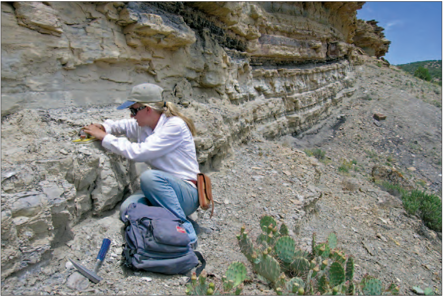
Shannon Townley, CGS mapping intern, takes a strike and dip reading on a bedding plane in the Dakota Sandstone near Delta. Photo by Dave Noe.
