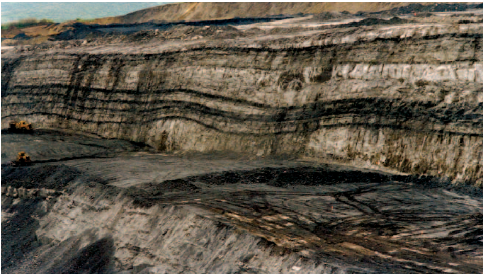
Figure 11. Cretaceous coal strata exposed in a bench cut of the Williams Fork Formation at the Kennecott Corp. Colowyo surface coal mine in Moffat County, Colorado. Note how the coal beds split and roll.
