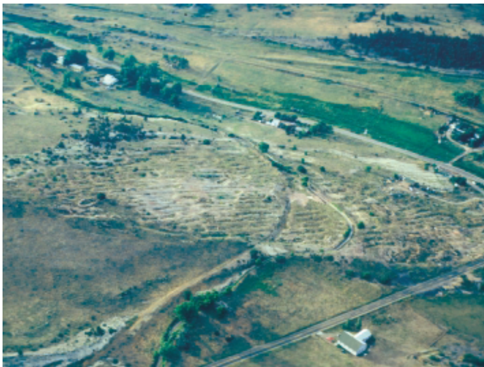
Subsidence into shallow abandoned coal mines near Marshall, Colorado
