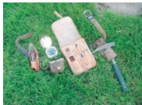
“Stuff” usually carried on a geologist’s field belt includes rock hammer, notebook case, Brunton compass, and hydrochloric acid. Photo by J. Keller.
