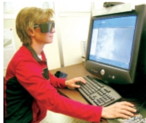
Geologist Beth Widmann wearing special electronic goggles that allow her to view aerial photographs in 3D on our mapping workstation. Photo by V. Matthews.
