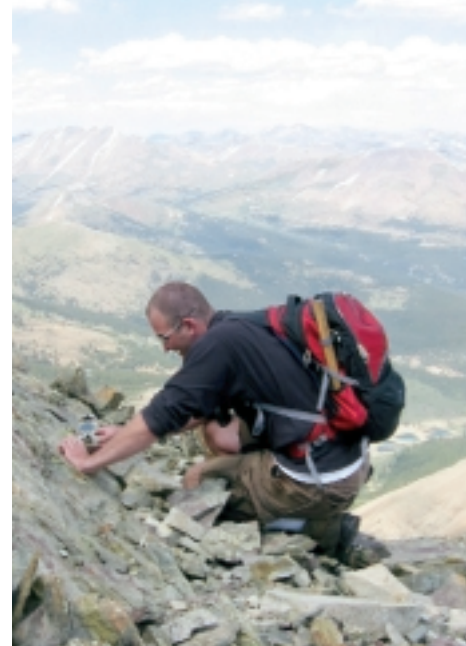
Field Assistant, Joel Poppert, measuring the tilt of bedding with a Brunton compass. Photo by Beth Widmann.
