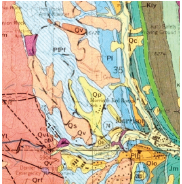
Geologic map of the area between the town of Morrison and Red Rocks Park. (from Scott, 1972). Each color represents a different rock formation or unconsolidated deposit occurring at the surface.
