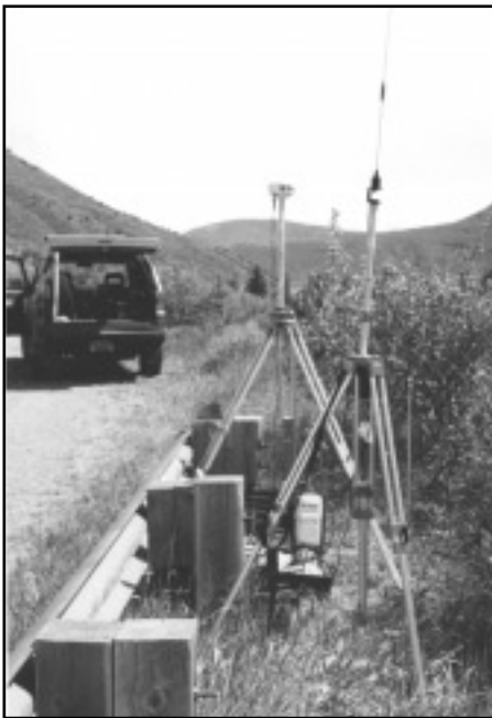
GPS technology is used extensively on Western Colorado projects for specialty survey and mapping work (This is a base station setup.)
