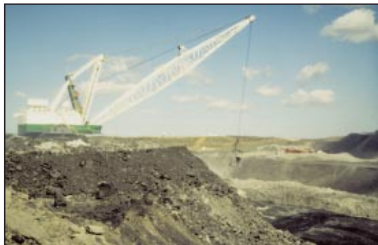
Dragline at Colowyo Mine with 60 cubic yard bucket capacity.
