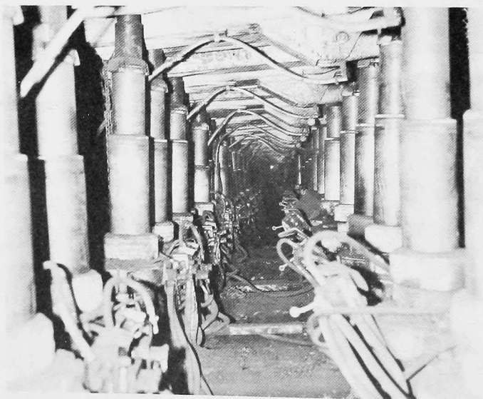
Figure 2. View looking down the chocks of a longwall unit showing the hydraulic roof supports. Each hydraulic leg has a 110-ton capacity, two-stage hydraulic extension.
