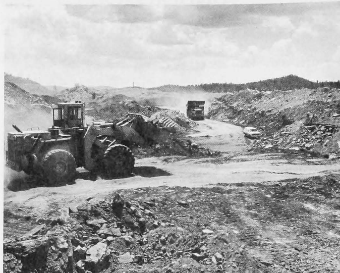
Figure 5. Fifteen-yard front-end loader awaits arrival of truck in the background to begin loading of overburden.
