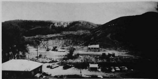
Figure 8. Andesite Rock Company quarry on South St. Vrain Creek southeast of Lyons. This rhyodacite sill intrudes east (left)-dipping sandstones and dark shales of the Pennsylvanian Fountain Formation. Photo by James Soule, Colorado Geological Survey.
