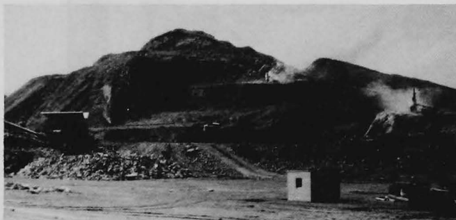
Figure 7. Working face at the new Ralston quarry, operated by Asphalt Paving Company. The company currently produces dark-gray monzonite from the oval-shaped intrusive at a rate of 3000 ton/day for use as road base and concrete and asphaltic aggregates.
