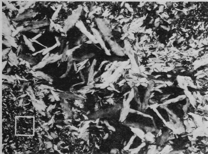
Figure 7. Photomicrograph of same specimen as in Figure 6. Coarser elongate alunite crystals (light) and microquartz (dark) metasomatically replacing feldspar phenocryst in quartz-lattice porphyry. Crossed polarizers. Square 0.1 mm across.
