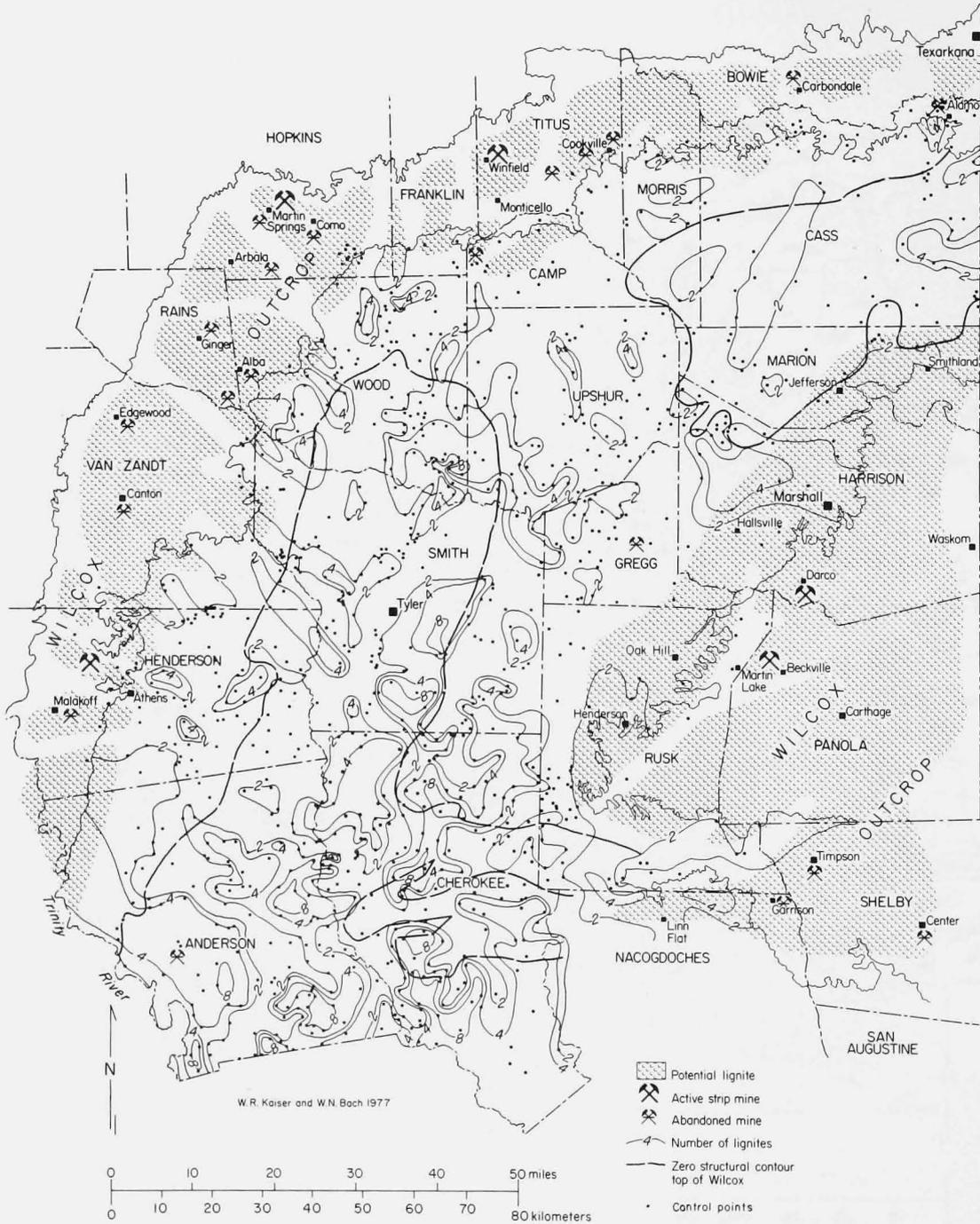
Figure 13.--Occurrence of lignite in the undivided Wilcox Group.
