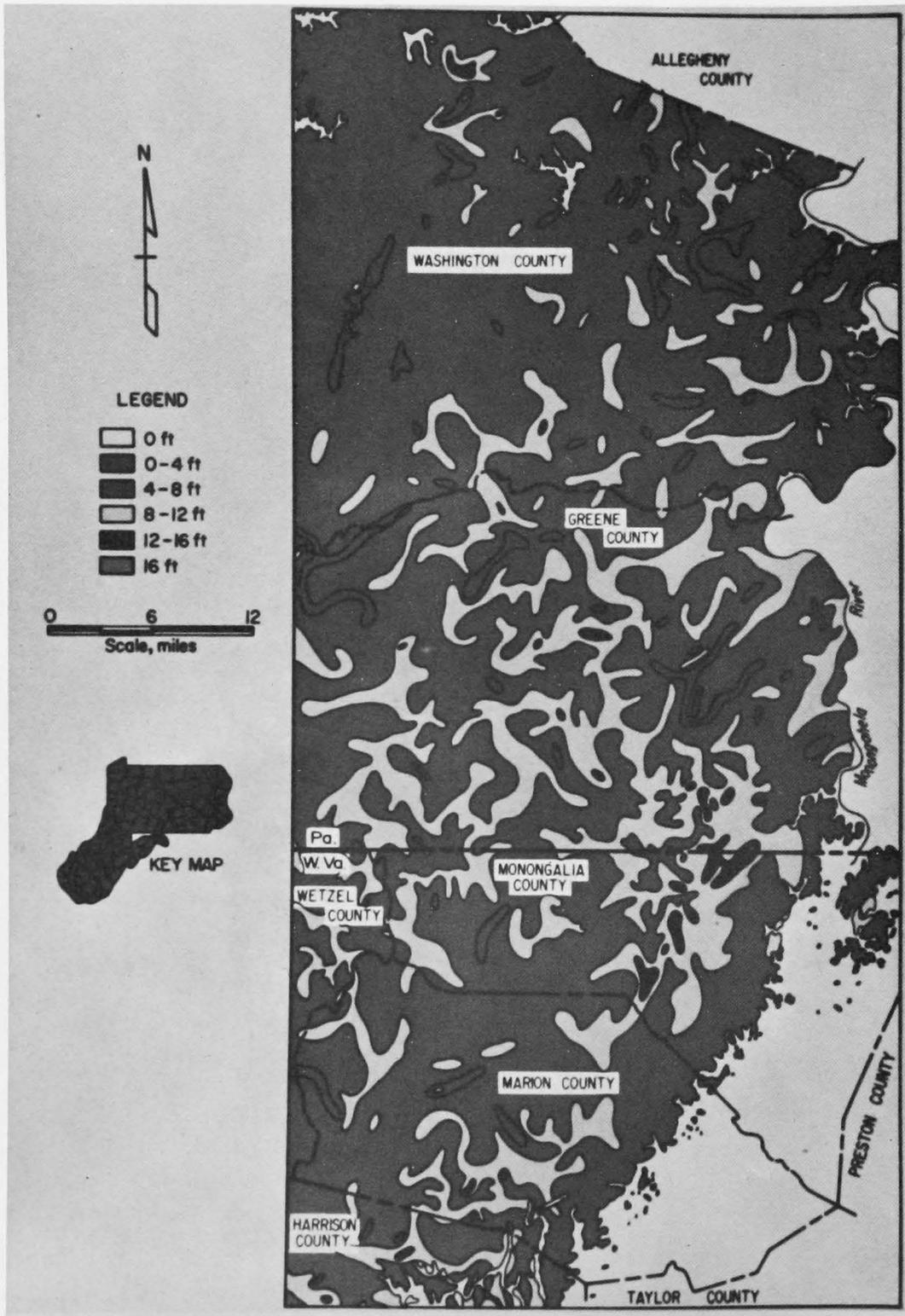
Figure 23.--Isopach of Pittsburgh coal. Modified from McCulloch, Diamond, and others, 1975.
