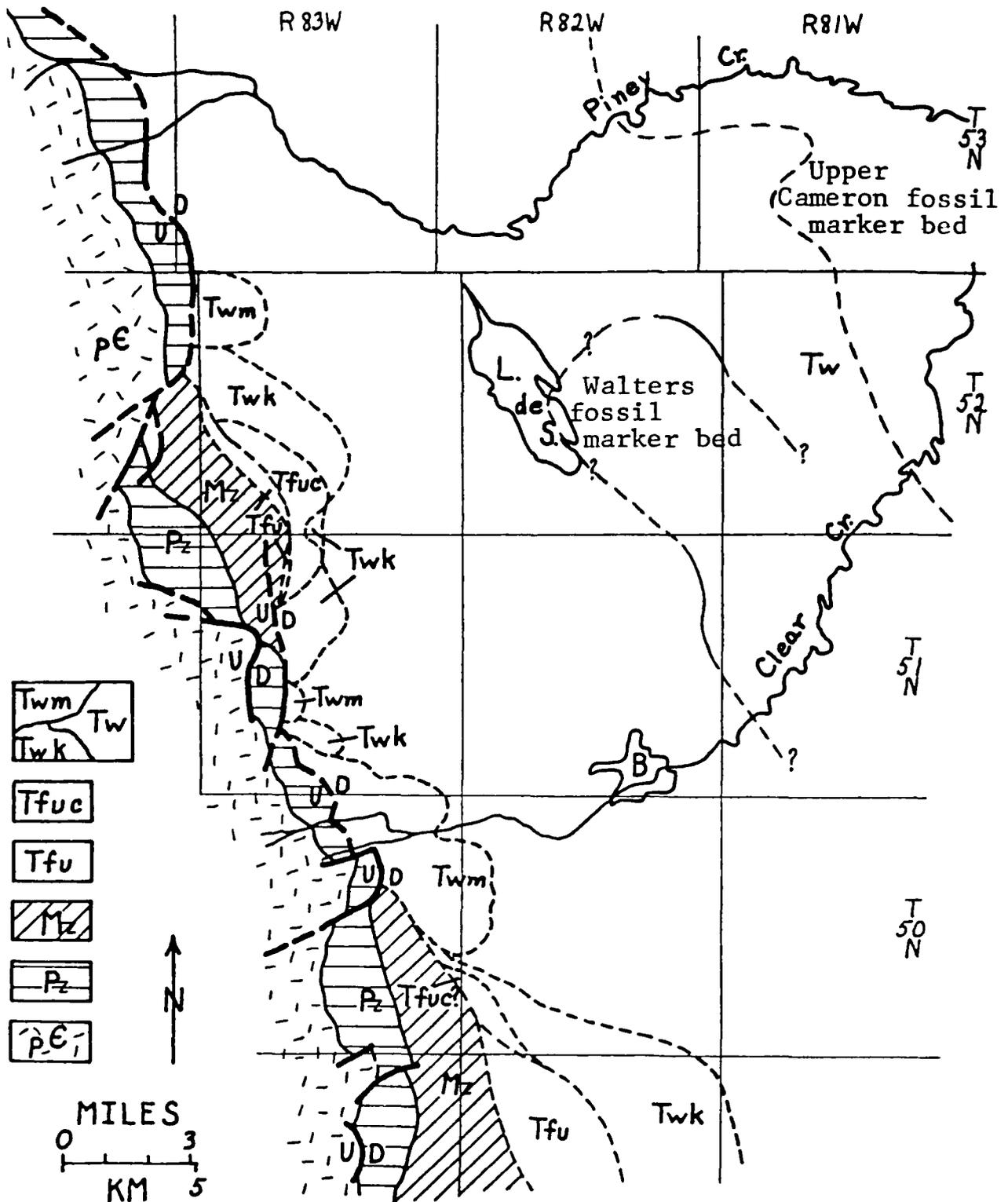
Figure 9.--Areal extent of the fossiliferous marker beds located above the Upper Cameron and Walters beds. pE, Precambrian; Pz, Paleozoic units, undivided; Mz, Mesozoic units, undivided; Tfu, Ft. Union Formation; Tfuc, Conglomerate Member of the Ft. Union Formation; Tw, Wasatch Formation; Twk, Kingsbury Conglomerate Member of the Wasatch Formation; Twm, Moncrief Conglomerate Member of the Wasatch Formation. Geology modified from Mapel (1959) and Hose (1955).
