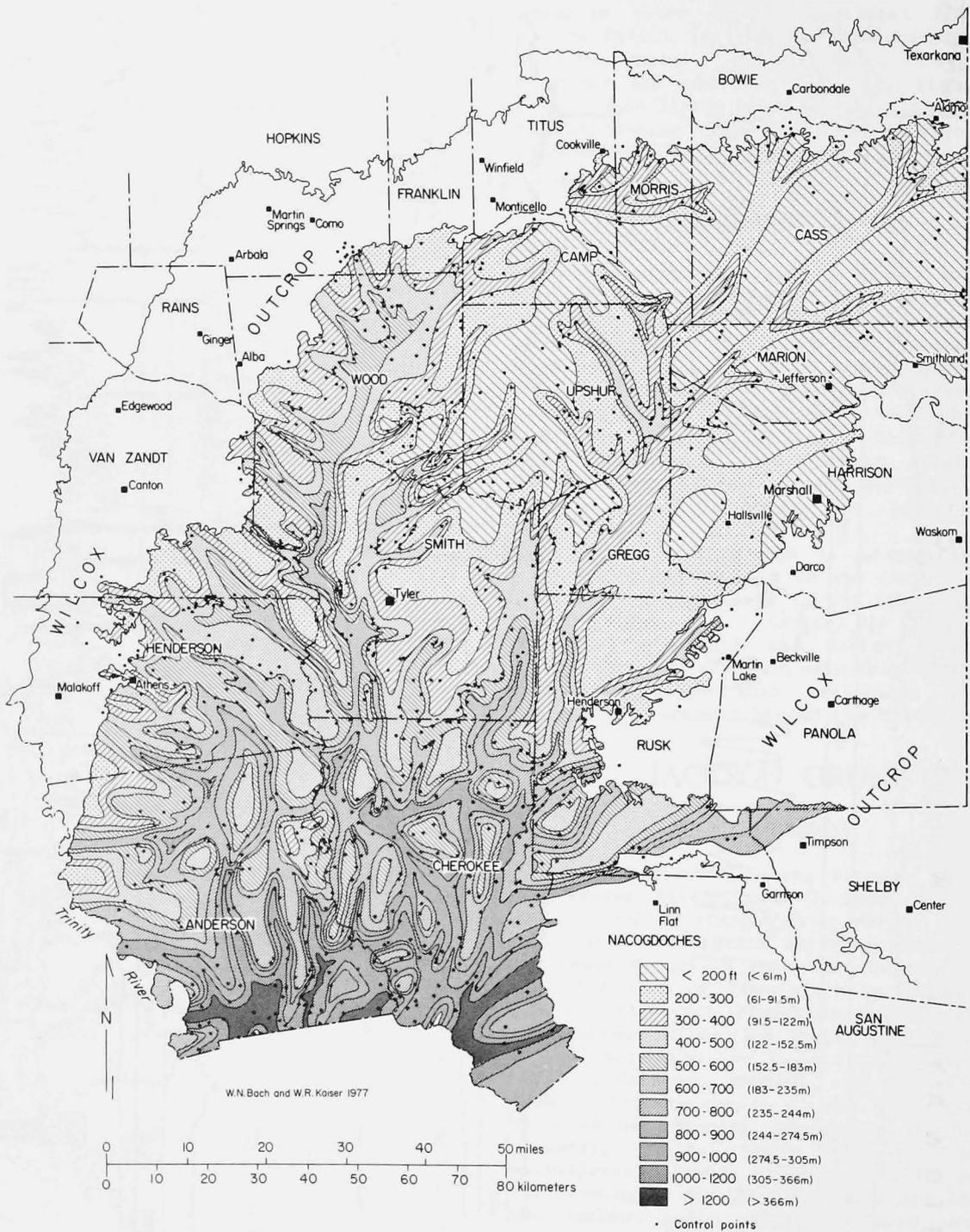
Figure 11.--Net-sand map of the undivided Wilcox Group. Wilcox outcrop from Barnes (1965, 1966, 1967).
