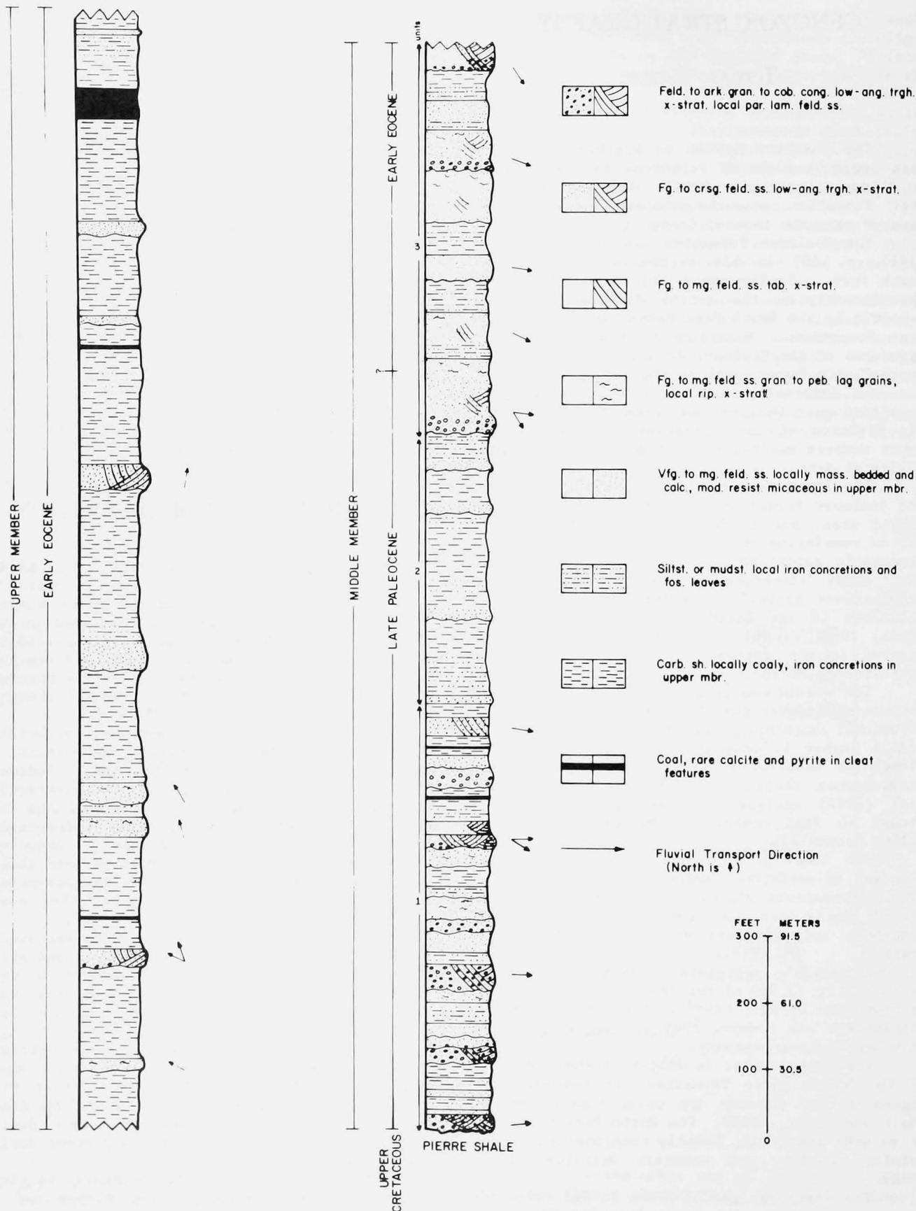
Figure 3.--Generalized composite stratigraphic section of the upper and middle members of the Coalmont Formation near Coalmont, Jackson County, Colo.
