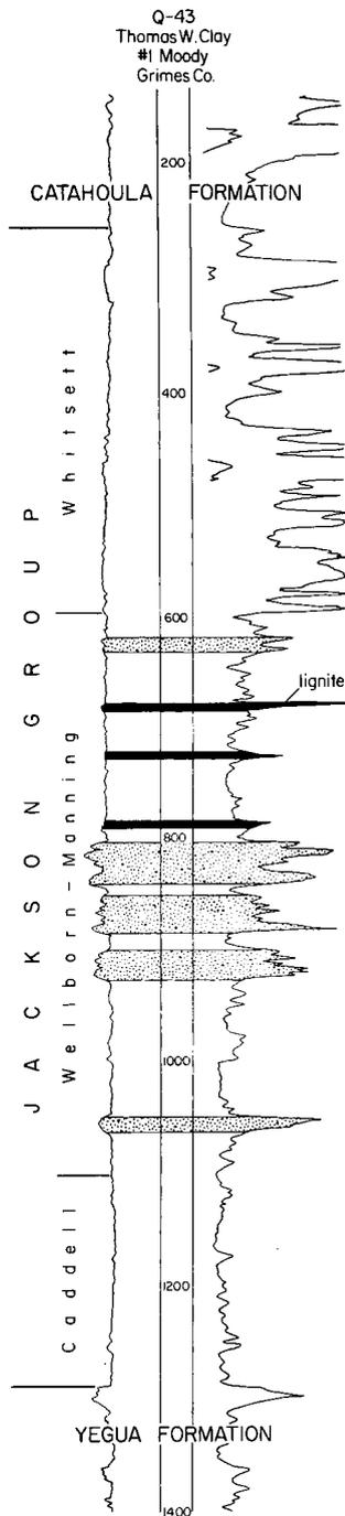
Figure 14.--Jackson stratigraphy of southeast Texas and the occurrence of lignite. See figure 15 for location of electric log.
