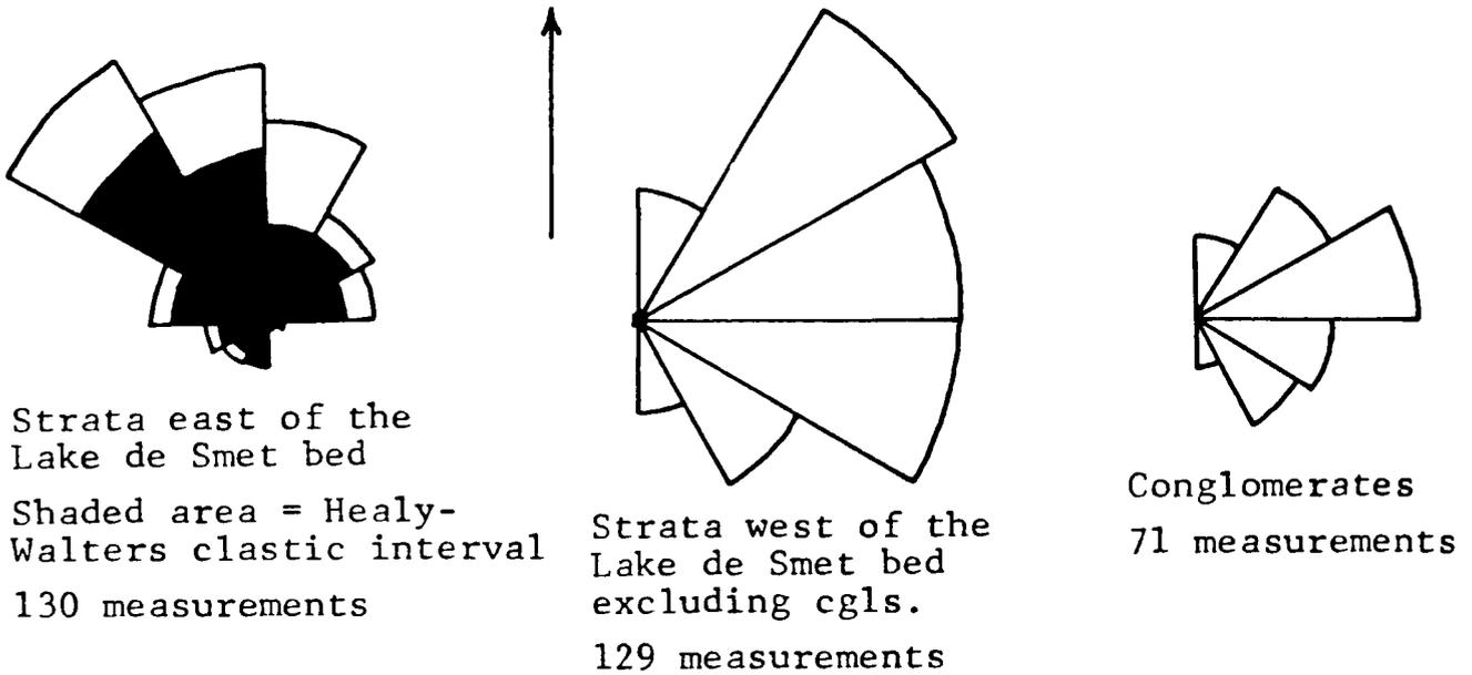
Figure 13.--Rose diagrams for transport directions in the study area.
