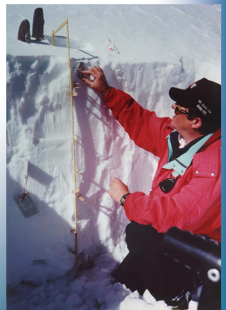
Checking snow crystal type and layer data from a snow pit
