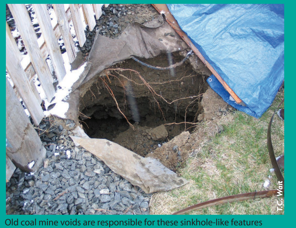
Old coal mine voids are responsible for these sinkhole-like features
