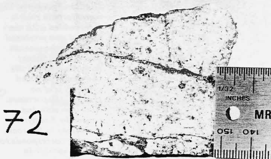
Figure 4: Pyrite disseminated in granodiorite of the Oligocene White Rock pluton. Sample was taken from south of the Colorado-Highland Claim block. Samples taken from this area contain no economic values in gold or silver. Number corresponds to sample collection number. See Appendix A.
