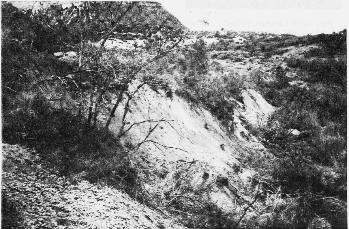
Figure 19. Scarp exhibiting about 20 feet of vertical displacement crosscuts the slide mass approximately one third of the distance up the slide from the toe. Refer to Figure 18 for location.
