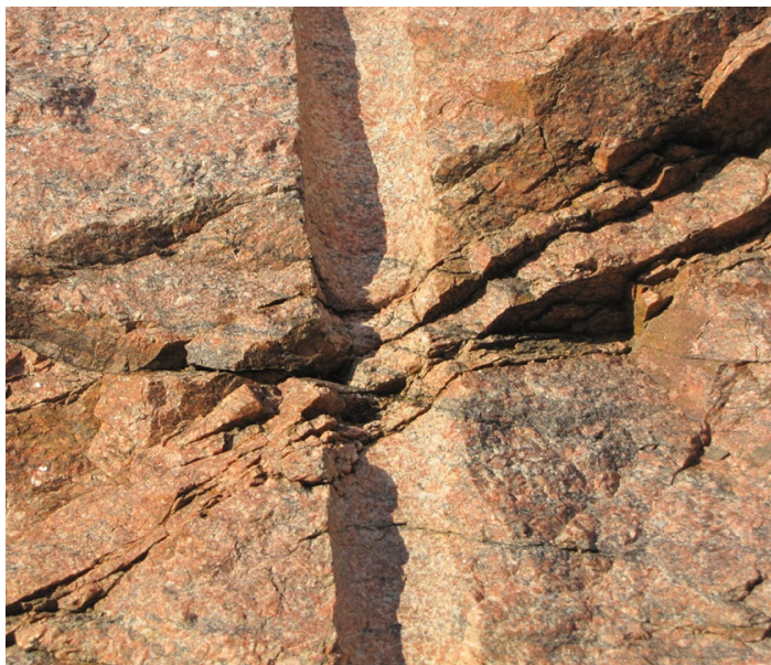
Fractured, crystalline bedrock, which is mostly massive granitic rock or banded gneiss, makes up the primary aquifer in the foothills. The rock itself has no significant pore space between crystal grains to hold water; instead, water moves through open fractures. In this photo, a borehole drilled for blasting to widen a roadway cuts through granitic rock, illustrating what a well would look like viewed from underground. In this example, the borehole hole intersects several fractures that could carry water.
