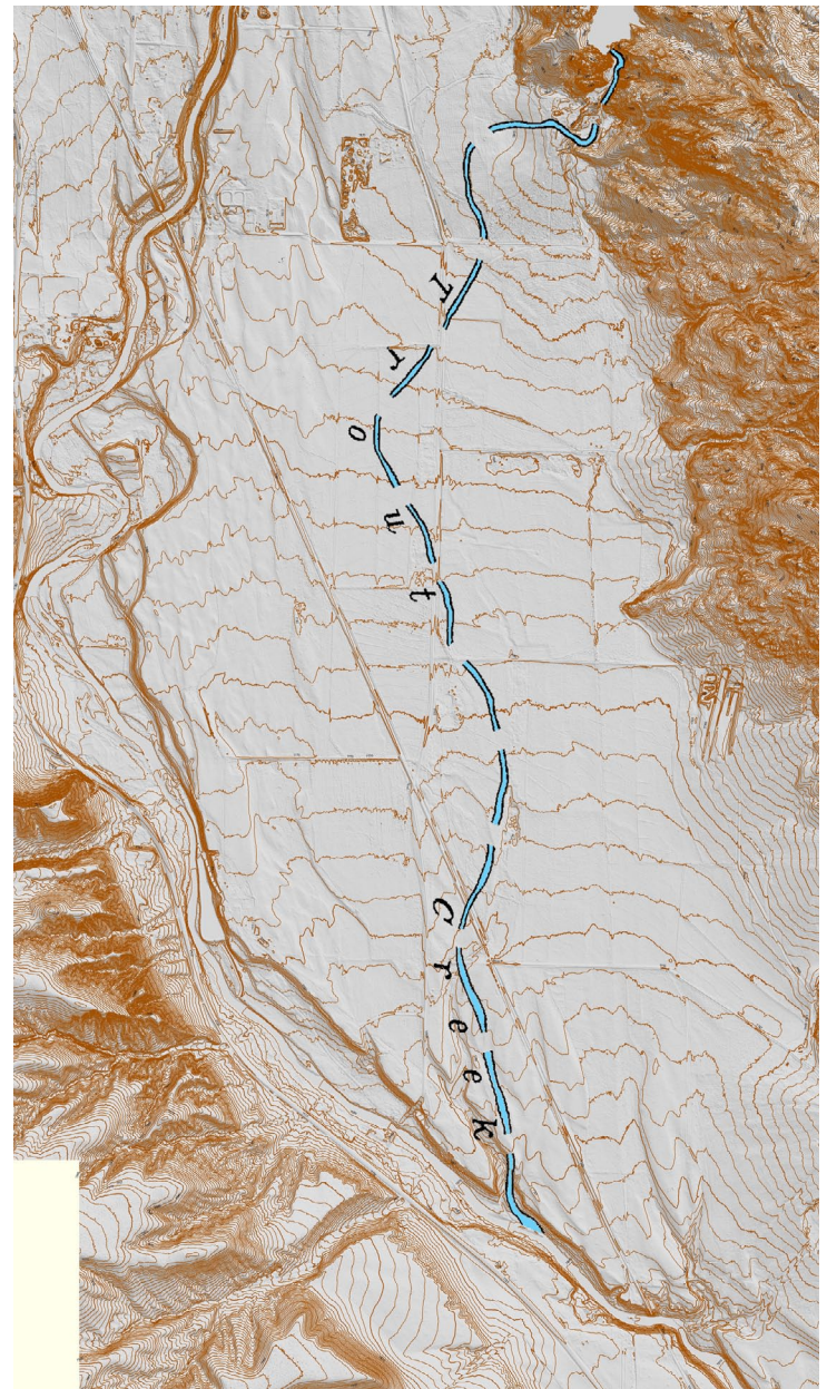
Figure 10 – Flood deposits from Trout Creek spread out over the Arkansas Valley floor to produce a very flat surface sloping to the south. Contour interval is 5 ft. Ancestral Trout Creek c. 1884 from Poor, 1976, base map by author.
