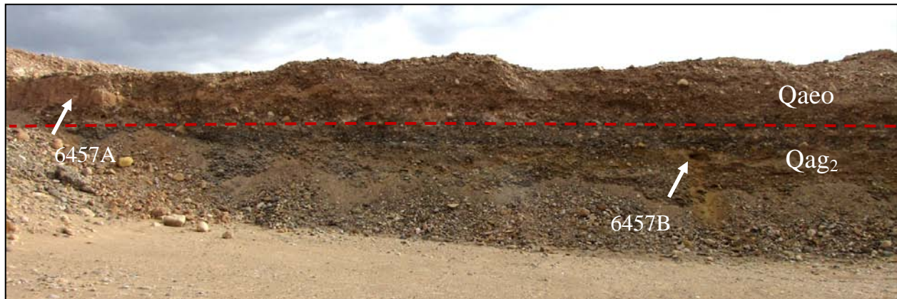
Figure 5. Quarry excavation in Gunnison River Qag 2 terrace overlain by Qaeo deposits sourced from East Creek of Unaweep Canyon. White arrows show sample location submitted for OSL dating (Appendix B) [UTMX 200440, UTMY 4320360].
