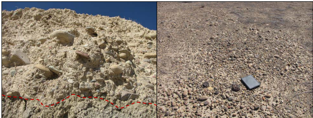
Figure 9. Old gravel deposits ( Qgo ) overlying weathered Mancos Shale. Contact is shown by dashed red line. Note the deposit is poorly sorted but clast imbrication can be seen [UTMX 202530, UTM Y 4322030]. Photo on left shows surface of deposits where finer-grained matrix has washed away leaving an armored surface of cobble to pebble sized gravel [UTMX 202820, UTM Y 4322270].
