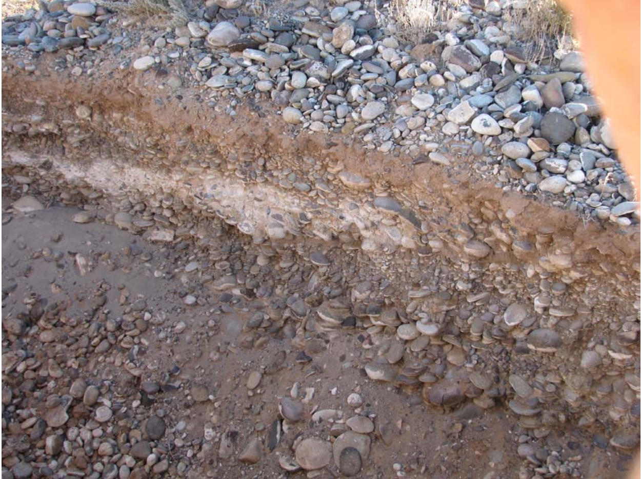
Figure 4. Prospect pit excavated in Qag 4 deposit. Note calcic soil development [UTMX 199390, UTM Y 4320120].
