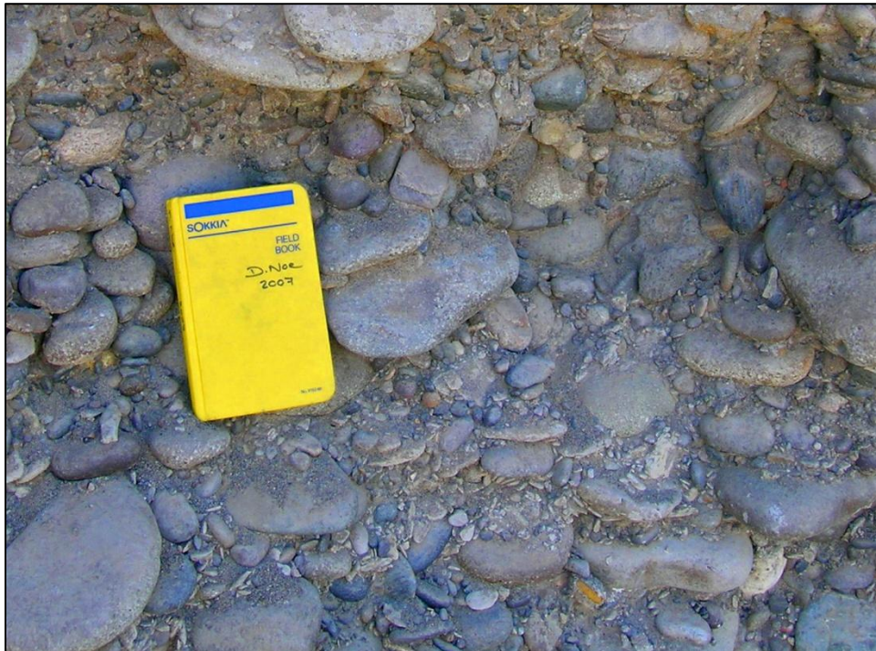
Figure 5. Alluvium four of the Gunnison River ( Qag 4 ), exposed in the wall of a gravel pit. The deposit consists of monochromatic, grayish pebbles and cobbles in a coarse-sand matrix. Compare this with the multi-colored Uncompahgre River gravel in Figure 3 . [UTMX: 239,690, UTM Y:4,293,223 ]
