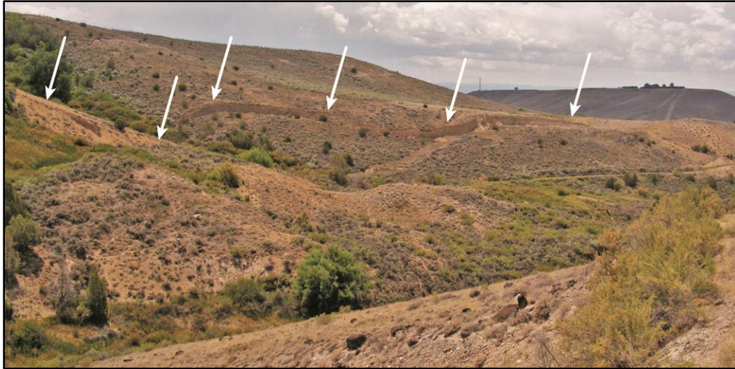
Figure 14. Large, recent landslides on Redlands Mesa along Currant Creek, near Madison Gulch. These landslides were initiated by the cutting of an irrigation canal across the lower slopes, and by subsequent wetting of the slope by water from the unlined canal. A remnant of the now-abandoned canal may be seen in the middle right. The tops of fresh head scarps are marked by white arrows. The entire lower slope is failing and moving. [UTMX: 247,511, UTM Y: 4,303,250]
