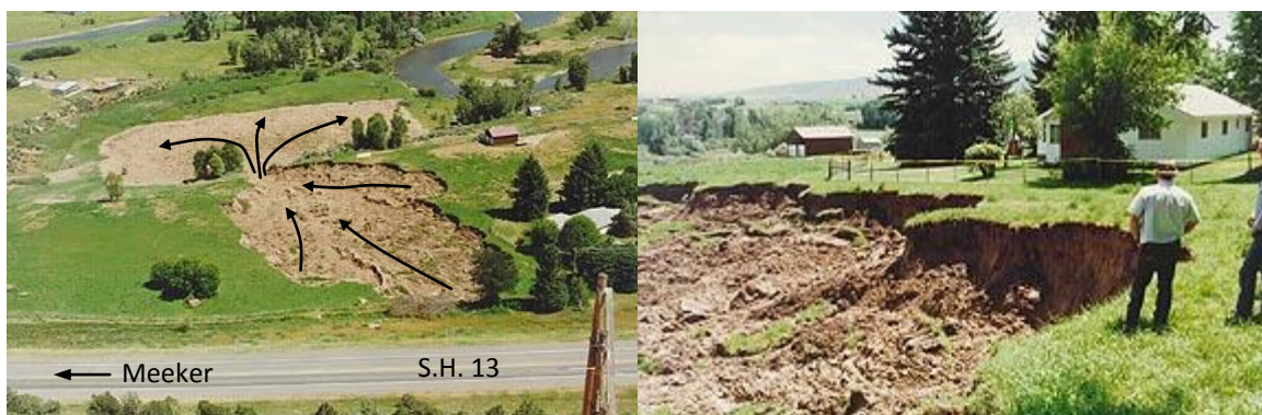
Figure 22. Earthflow of unconsolidated alluvial-fan soil near Meeker in 1996. Scarp is at irrigation ditch. Cause was over-irrigation and saturation of slope near river-meander bluff. Note the throat of failure where the bluff failed, mobilization and flowage of soils occurred towards it, and the resultant mud fanned out over the lower field adjacent to the White River. [UTMX 249177, UTM Y 4434934]
