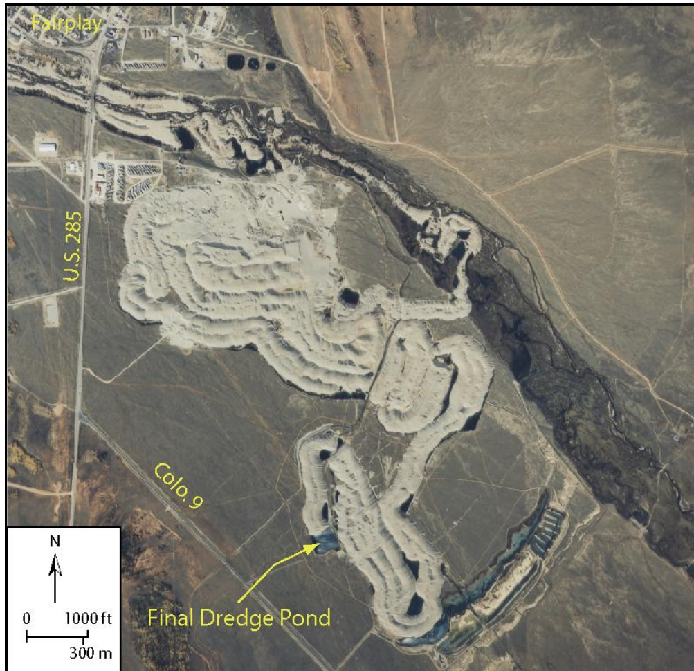
Figure 4. Aerial photograph of mine waste piles southeast of the town of Fairplay. Local residents refer to the sinuous and looping piles as the “intestines”. The final dredge pond marks the last pond in which the dredge boat worked. (USDA photograph 612120 2495-124; flown September 29, 1997)
