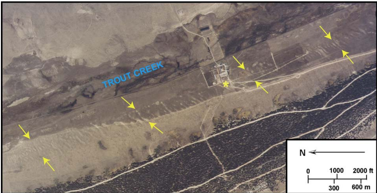
Figure 11. Aerial photograph of Trout Creek valley. North is to the left. Note the narrow linear belt of short, northeast-trending, subparallel ridges and swales, which is outlined by the yellow arrows oriented parallel to the ridges and swales. The belt of ridge-and-swale topography trends north-northwest, parallels the strike of Mesozoic bedrock in the area, and is over 3 miles long. A yellow asterisk marks the pit in which Oligocene sedimentary rocks are exposed. (U.S. Bureau of Land Management photograph, project CO-81CC, frame 11-35B-10; flown October 6, 1982)
