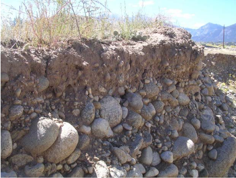
Figure 8. Older Pinedale outwash gravels (Qpoo) underlying a terrace on the western side of the Arkansas River, north of Buena Vista (Sec. 5, T14S, R78W). Photo shows the south wall of the Hard Rock Paving gravel pit. Note weak surface soil developed in sandy sediments overlying the cobbly channel gravels.
