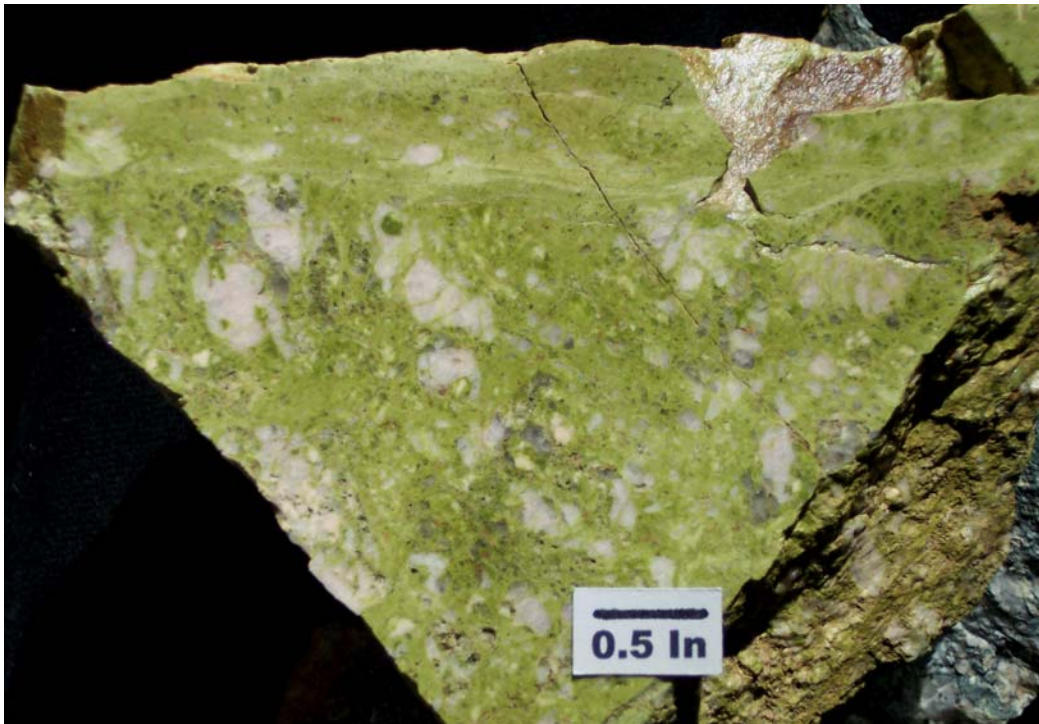
Figure 35. Laramide (?) epidote-matrix fault breccias in Proterozoic rocks on the east side of the rift, northeast corner of the Buena Vista West quadrangle.
