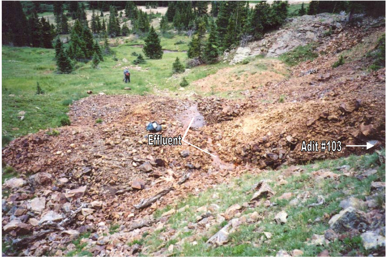
Figure 9. Waste-rock pile and effluent from adit #103.
