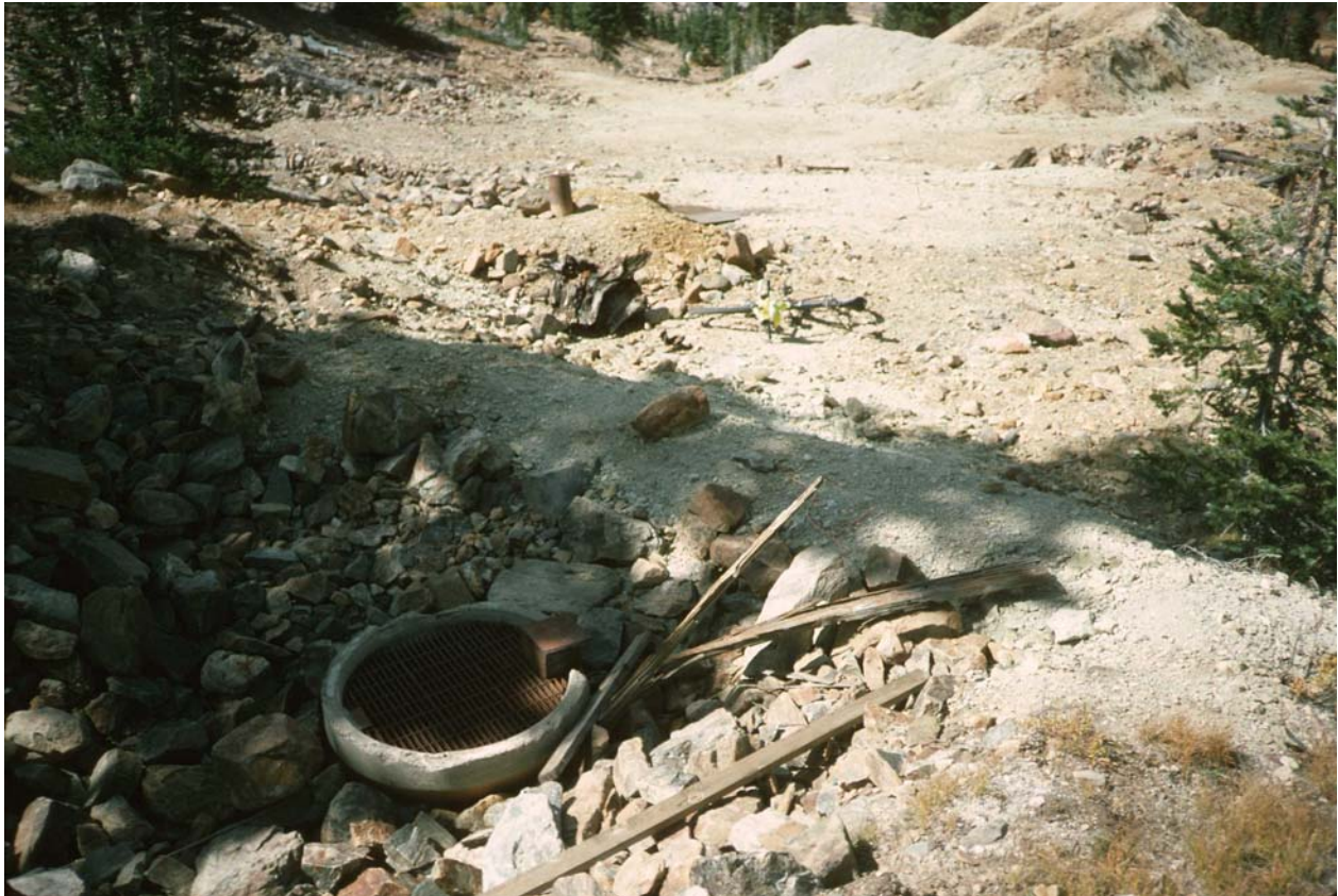
Figure 48. Close-up view of grated effluent inlet, Pennsylvania Mine-level F (#100). Photo taken Sept, 1993.
