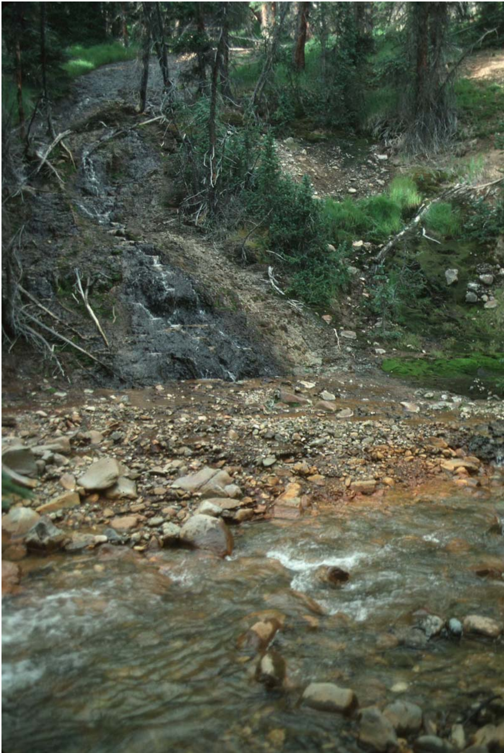
Figure 11. Pass-Me-By Mine effluent entering Iron Creek.
