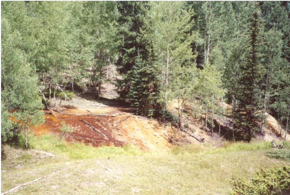
Figure 33. Iron-hydroxide precipitate and filamentous algal growth near portal of Ferricrete Mine adit.
