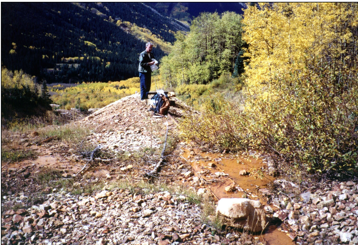
Figure 14. Effluent braiding on bench of dump #201.
