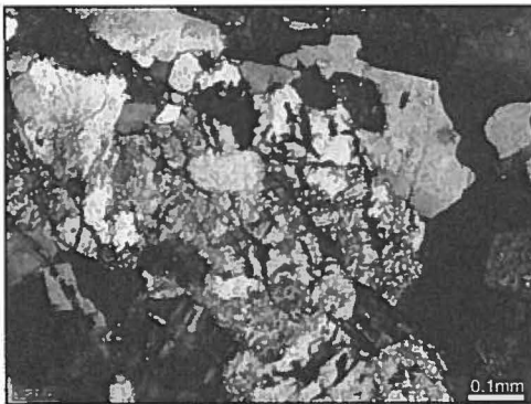
C. Sample NE9, biotite gneiss from north-eastern transect. Brittle deformation and strong sericitization (brown).
