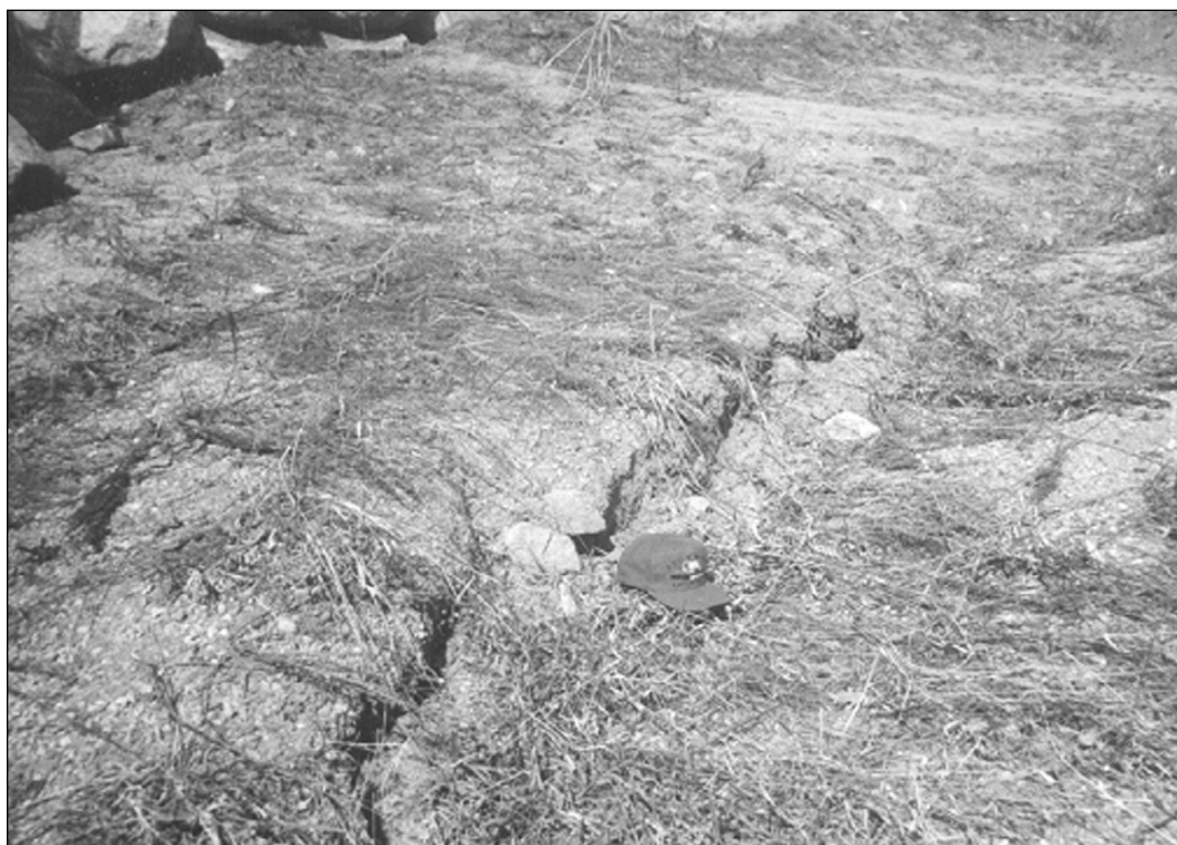
Figure 5. Ground crack and beginning of landslide scarp in the Broadmoor area in 1998. Note hat for scale. Photo by J. White.
