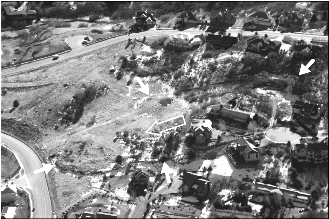
Figure 8. Regency Landslide in the Broadmoor area. White arrows delineate landslide boundary. Hollow arrow points in the movement direction. One home near head scarp that is shown below was condemned and demolished before this photo was taken, only broken foundation and driveway from cul-de-sac show on this photo. Note landslide toe formation in small field near lower road. Photo taken in 1999 by M. Squire.
