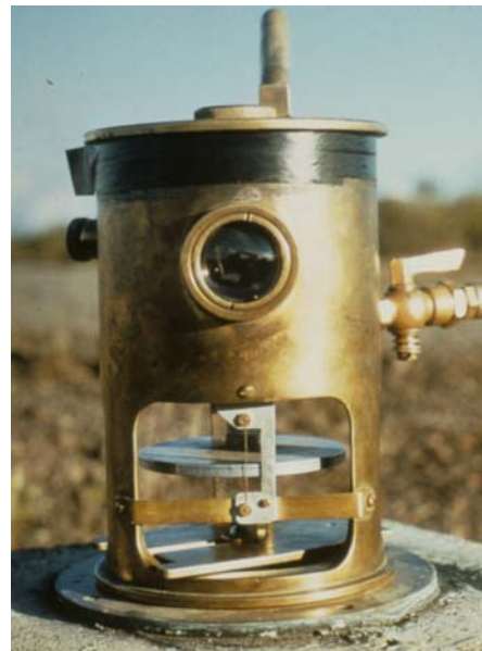
Sensitive instruments, like this tiltmeter, help to provide warnings that prevent loss of life from volcanic hazards. Instruments can help geologists keep watch on areas of concern, some of which are listed in the table on the facing page. (photo by J. C. Ratte from USGS photo library)
