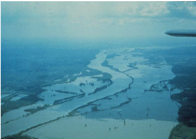
Flood plains of major rivers experience frequent flooding. This aerial view shows spring flooding of the Missouri River downstream from the mouth of the Osage River junction in April of 1973. Floodplains that are inundated frequently merit either flood control structures or limits on development. Reconstruction of flood-damaged homes on flood-prone sites using federal insurance claims payments results in a repeated drain on the flood insurance fund by a relatively small number of insured structures. (photo by Richard Waugh)
