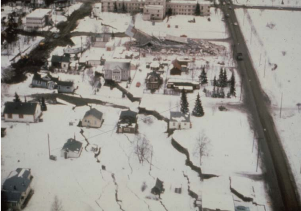
Low-altitude aerial photograph of Anchorage, Alaska, after the 1964 earthquake. Fissures at the head of landslide blocks can be seen passing through the Turnagain Heights neighborhood. The area between the major fissures dropped down as result of the consolidation and settling of porous sediments during the strong tremors. Ruins in background are remains of the Four Seasons apartment building. Landslides are a common product of earthquakes, and many slides close roads and delay rescue and repair efforts. (photo from USGS Photo Library, Denver, CO)
