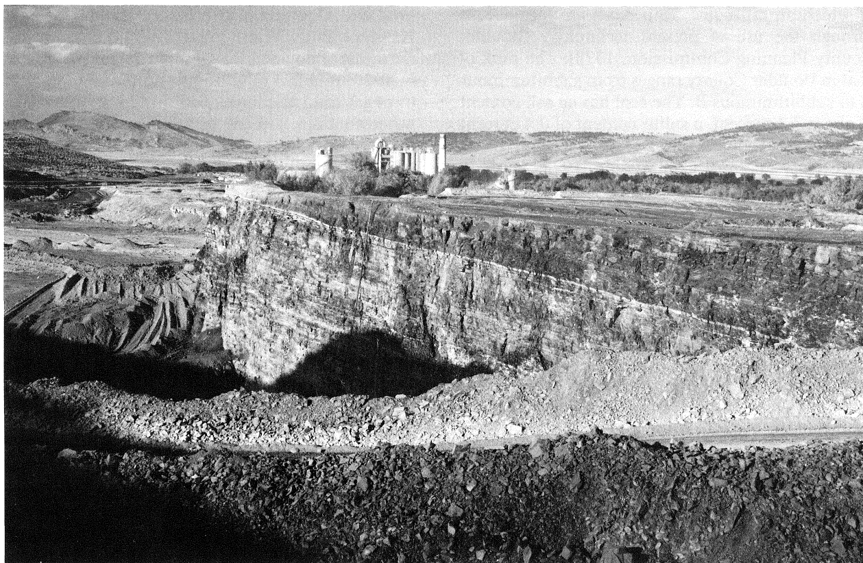
Figure 16. Martin Marietta cement plant in background, limestone quarry in Fort Hays Limestone member of the Niobrara Formation in the foreground; location 1 on Figure 1.
