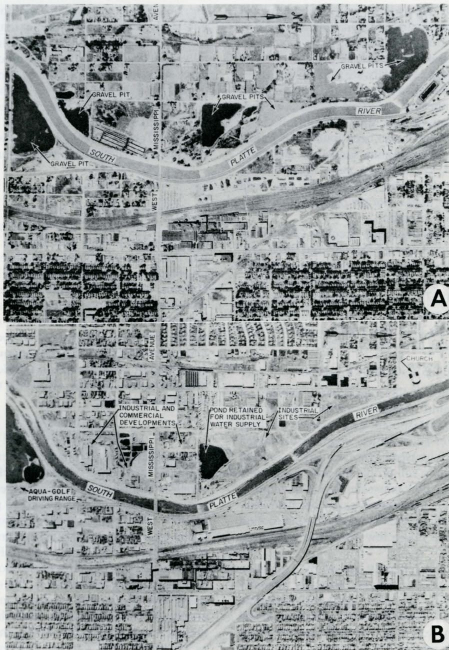
Figure 14. Airphotos of a reach of the South Platte River in Denver, (A) in 1949, and (B) in 1965 following filling of gravel pits with municipal wastes and subsequent urbanization (Sheridan, 1967). The location of the airphotos is shown in Figure 1.
