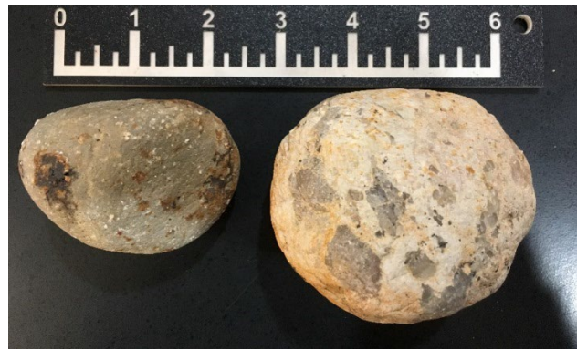
Fig. 29. Arapahoe Formation cobbles. Extrusive volcanic cobble (left) with tiny white crystals, and intrusive granite cobble (right) with large crystals. Scale in inches. From the outcrop at Fossil Trace Golf Course shown in Fig. 28.
