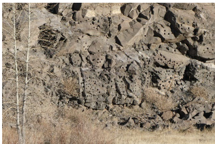
Fig. 94. Got holes? Drill holes in basalt cliff face of Quarry #2 left behind from testing in the 1960s. View to east.
