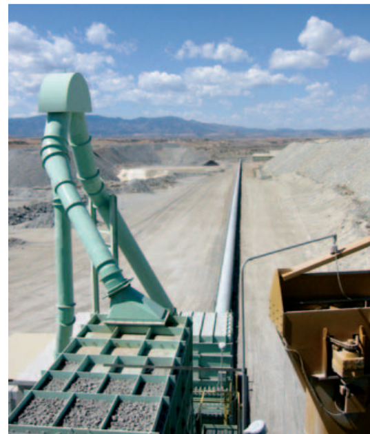
Figure 58. Primary crusher (foreground) and blending hall (at distance) at Holcim's Portland cement plant in Florence. The long belt connecting the two is necessitated to ensure proper blending of limestone, shale, and sandstone into a clinker mix in the blending hall.
