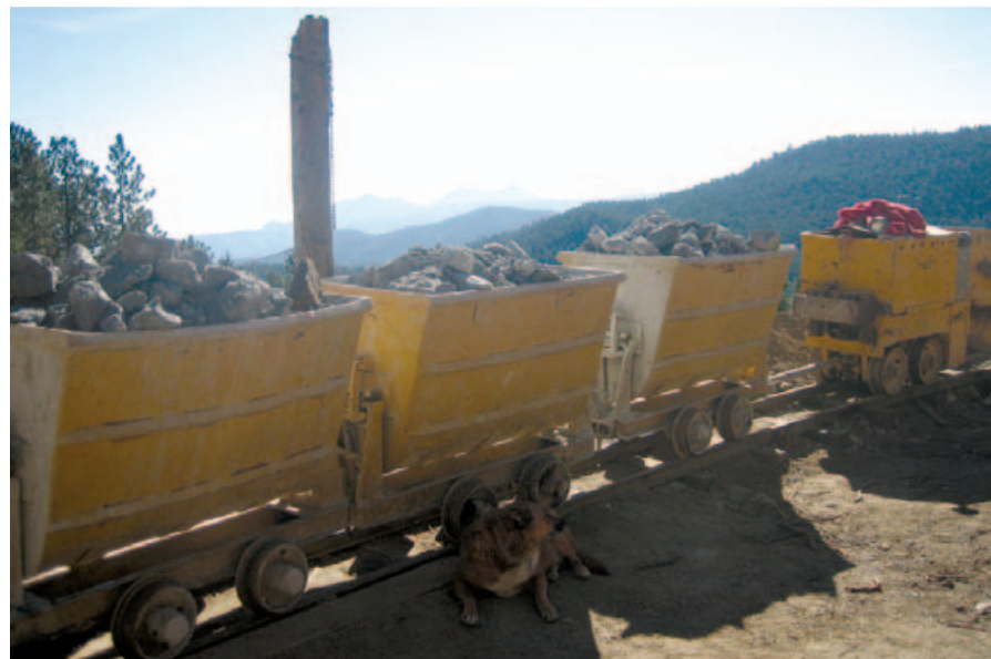
Figure 50. Ore cars at the Cash Mine. (Photo courtesy of Mont Royale Ventures, LLC.)
