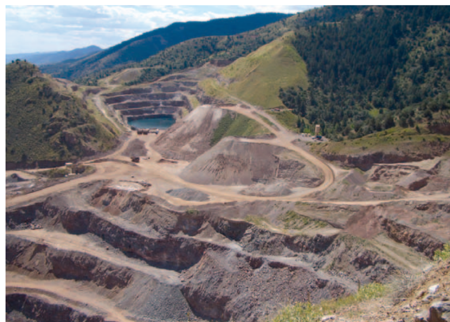
Figure 56. Precambrian metamorphic and granitic rocks are quarried at Aggregate Industries' crushed stone operation near the town of Morrison. View is to south (photo courtesy of Aggregate Industries).
