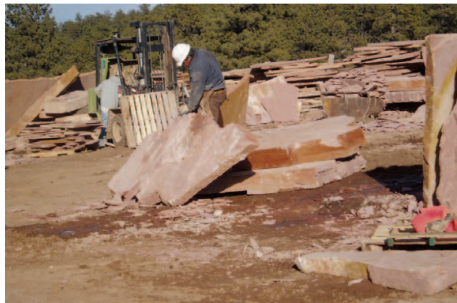
Figure 57. Workers hand-trim flagstone blocks at B&B Stoneworks' quarry near Lyons. The flagstone is derived from the Permian-age Lyons Sandstone.
