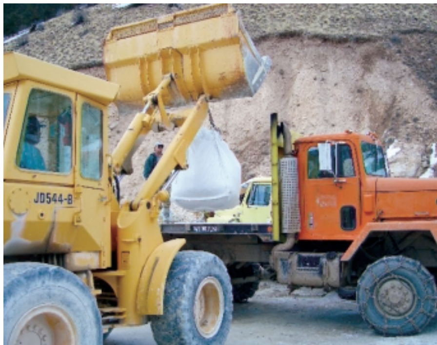
Figure 42. Loading a “super sack” of high-grade ore to a truck, Golden Wonder Mine, Hinsdale County. Ore from the mine is shipped to Nevada for processing; photo courtesy LKA International, Inc.
