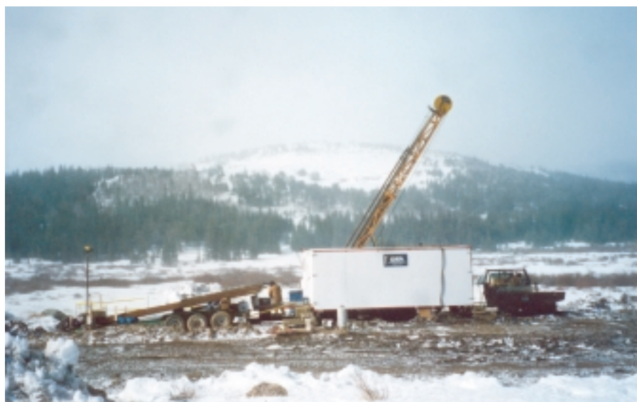
Figure 46. Angled core drilling on the No Name vein system, Caribou district, Boulder County. Drill is an Atlas Copco/Christensen QS 1000; photo courtesy of Tom Hendricks, Calais Resources Inc.
