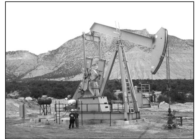
Figure 11. Surface pumping unit (pumpjack) on an Upper Cretaceous coalbed methane well. (Photo by Laura Wray)
