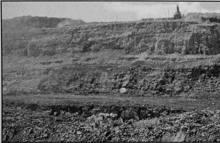
Figure 8. Colowyo's surface mine benching technique, Danforth Hills Coal Field, Moffat County.
