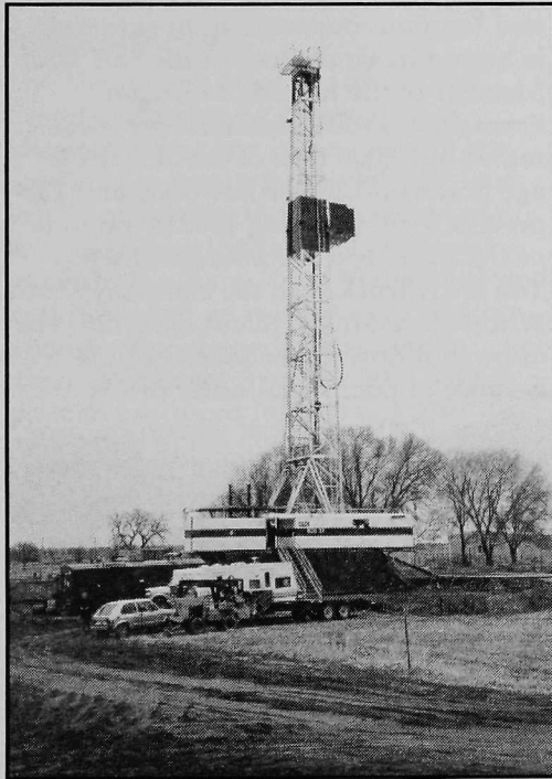
Figure 22. Caza Drilling Company Rig 17 on location in southwestern Weld County, April 2000. This H.S. Resources Incorporated well is scheduled as a 7,800 foot Muddy (J) Sandstone development well on the western edge on the Denver Basin's giant Wattenberg gas field.
