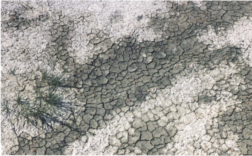
Shrinkage cracks form in expansive soils. Sulfate salts which are detrimental to concrete and metal leach out of corrosive soils.
