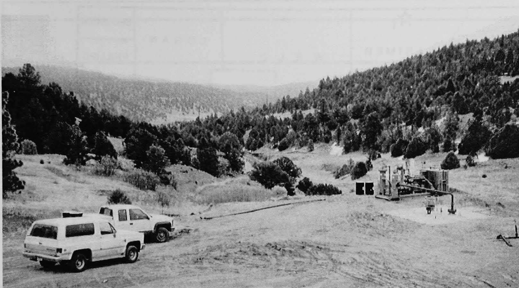
Figure 25. Stroud Oil Properties' recent Golden Eagle Mine vent hole completion in the Apache Canyon field, Las Animas County. In March 1997, this vent hole was producing about 350 thousand cubic feet of coalbed methane gas per day into the Colorado Interstate Gas Company Picketwire Lateral. Approximate depth to the Raton Formation Maxwell coal seam, which provided this gas flow, is about 300 feet below ground surface at this location.
