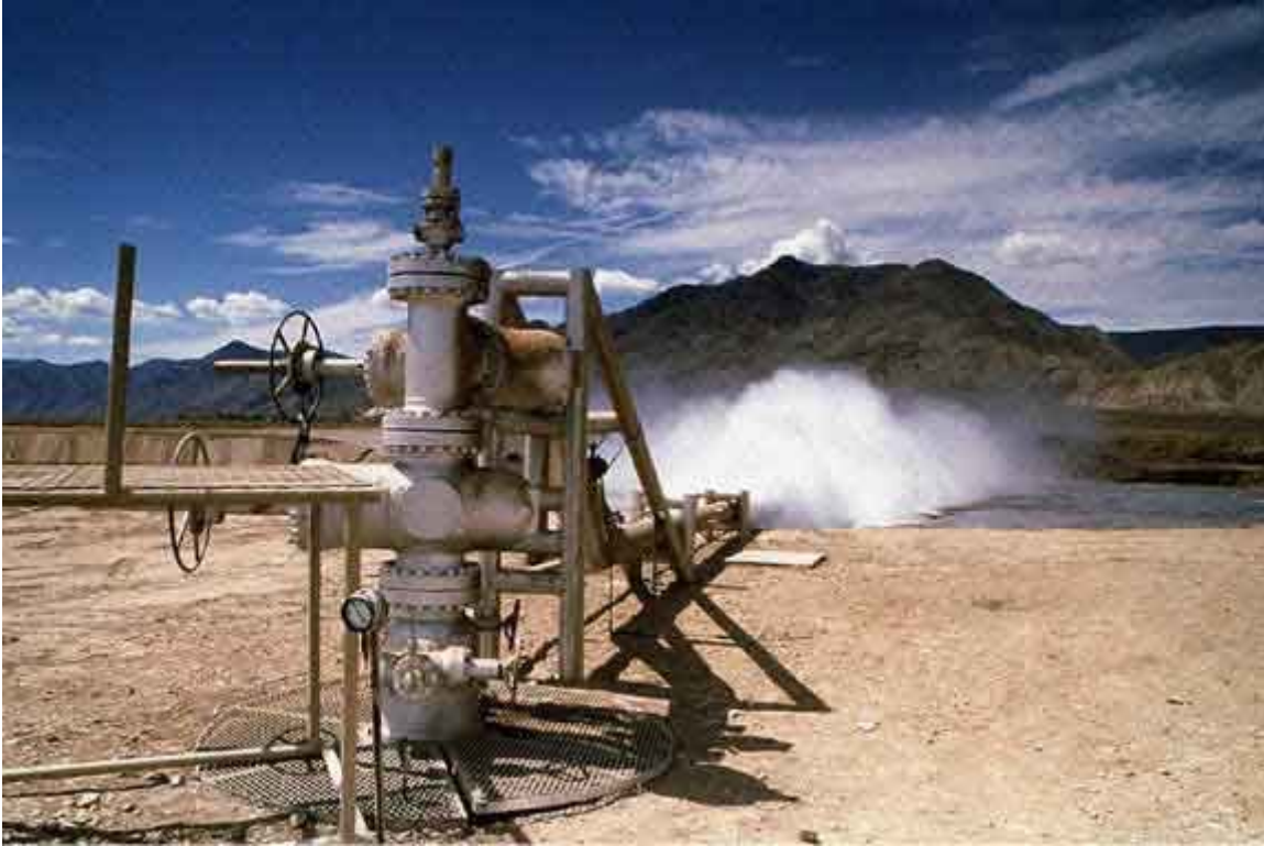
Flow testing of a reservoir after drilling. 11
