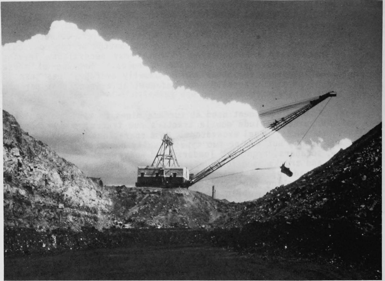
Figure 42. Photograph of a drag line, at a coal strip mine in Routt County, Colorado. (photograph by J. M. Soule)
