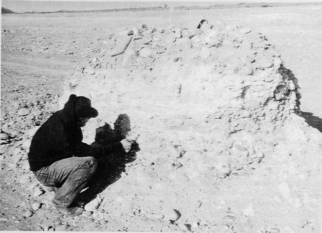
Figure 5. Terrace gravel of unit mtg in an excavation on Graham Mesa, near Rifle. Gravel is slightly cemented with pedogenic \text{CaCO}_3 and contains 20 to 30 percent grusified granitic clasts.
