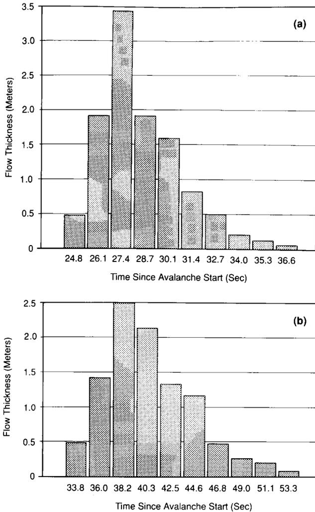
**Figure 23.** "Flow thickness" time distributions at the beginning of segments 8 (a) and 10 (b), Capitol Creek 2 avalanche, as computed from the particle model (Perla et al. 1984). Although the particle model does not compute flow thickness,  $d$ , this can be computed at any point on the profile by equation (3.26). Note lesser maximum thickness and longer duration of flow in segment 10.
