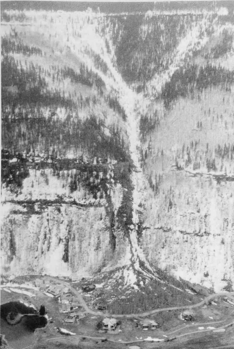
*Figure 26. Development along the perimeter of this alluvial fan in Vail, Colorado avoids the area of high avalanche pressure potential and frequency. Some of the homes are located within the Blue (moderate hazard) avalanche zone, and have been reinforced for design-avalanche loads. Compare this with pre-development photographs (Figures 17 and 18).*
