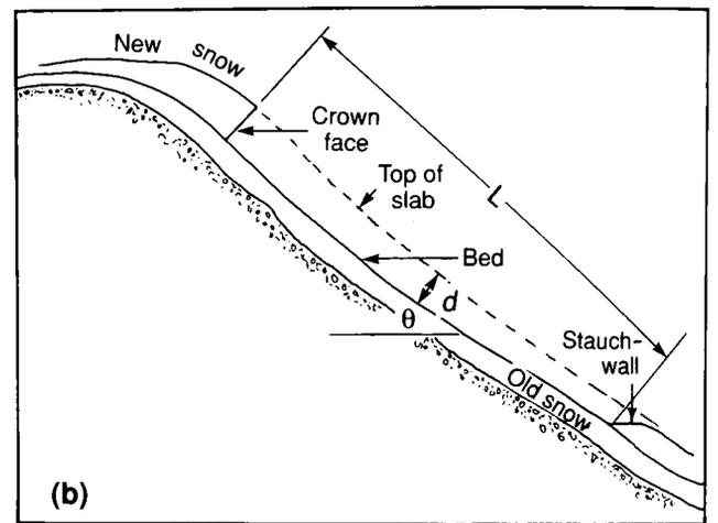
Figure 4. Terminology of a slab avalanche release, (a) plan view, and (b) elevation.
