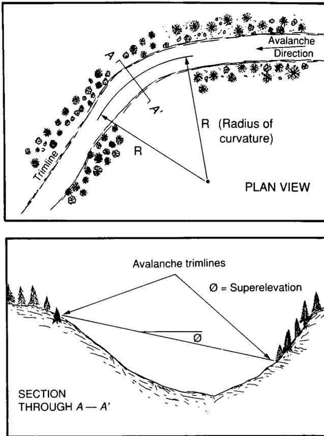
Figure 24. Superlevation measurements used in avalanche channel for velocity calculations.
