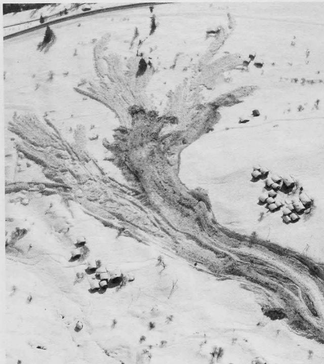
**Figure 12.** Runout of a large, wet-snow avalanche onto a populated alluvial fan in Switzerland. Debris advanced for long distances as sliding, reaggregated blocks of wet snow. Photograph was taken by the Swiss Army, and supplied by the Swiss Federal Institute for Snow and Avalanche Research.
