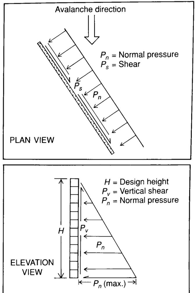
Figure 30. Forces acting on an avalanche deflecting wall.
