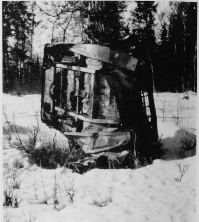
*Figure 10. Effects of powder-avalanche blast at the "Van Slide," south central Alaska. Powder blast wrapped this unoccupied vehicle, which was parked approximately 10 m upslope, around a cottonwood tree. Flowing-avalanche debris did not reach the tree, however vegetation damage occurred over 100 m downslope.*
