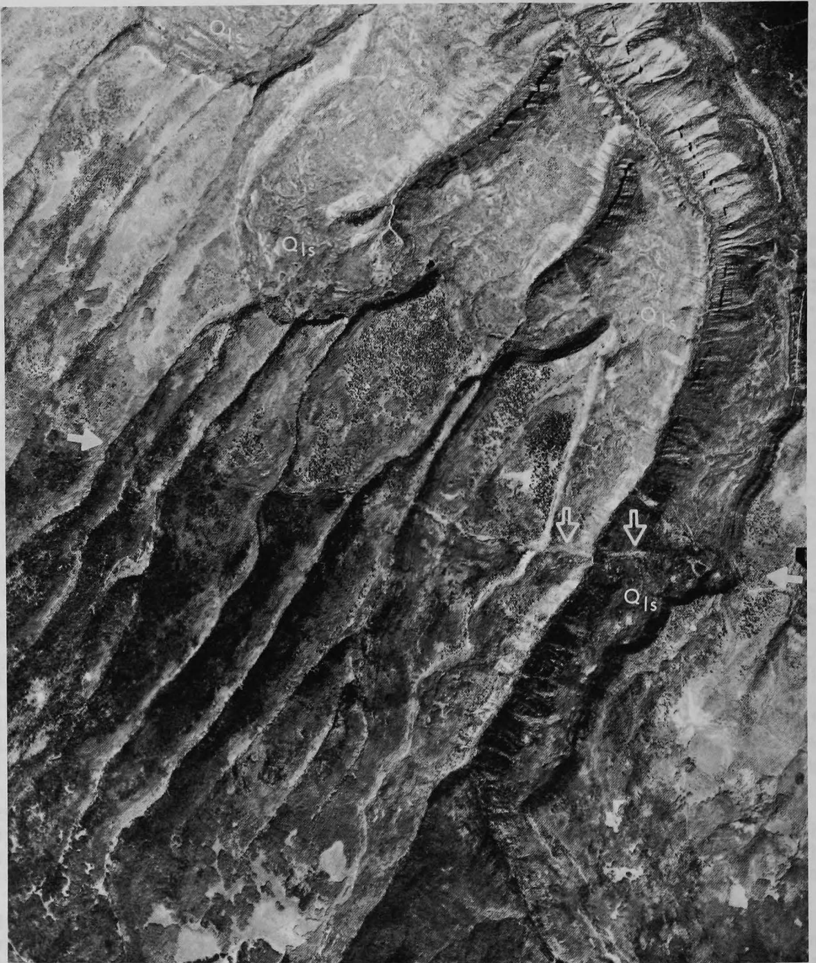
Figure 40. Vertical aerial photograph of fault 82 (solid arrows) where it crosses Roubideau Creek. Note hummocky landslide-covered terrain (Q1s) on the Brushy Basin Member of the Morrison Formation. An apparent scarp (open arrows) is developed in these Quaternary landslide deposits along fault 82. (photograph by Army Map Service; held by U.S. Geol. Survey)
