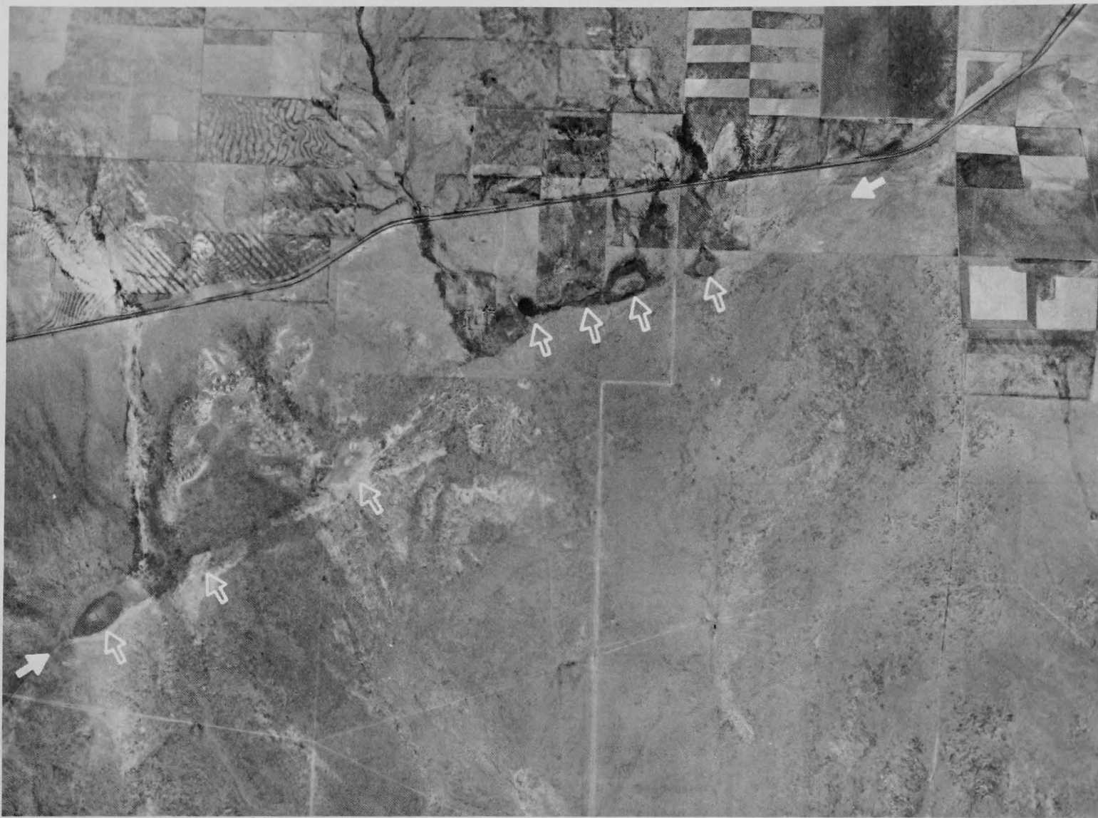
Figure 35. Vertical aerial photograph of part of the Cheraw fault. Note prominent sag ponds (open arrows) along fault scarp (solid arrows). (photograph by Army Map Service; held by the U.S. Geol. Survey)
