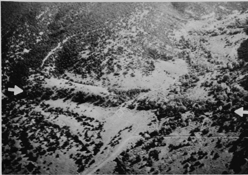
Figure 15. Oblique aerial photograph of the Sangre de Cristo fault at Uracca Creek. Note change in scarp height in alluvium of different ages. Arrows indicate scarp and diamond indicates location of truck shown in Figure 16.
