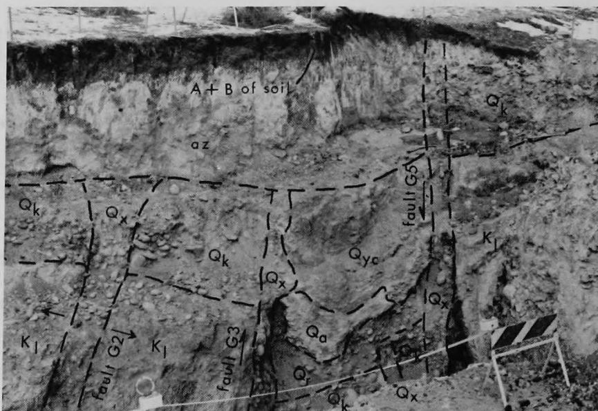
Figure 24. Photograph of the east side of the graben near Golden looking north (see Figure 23 for location of photograph). Note faulted Kansan(?) outwash (Qk), especially the 5.5 m offset along fault G5 and the zone of aligned gravel clasts (Qx). See Figure 21 for an explanation of the symbols.
