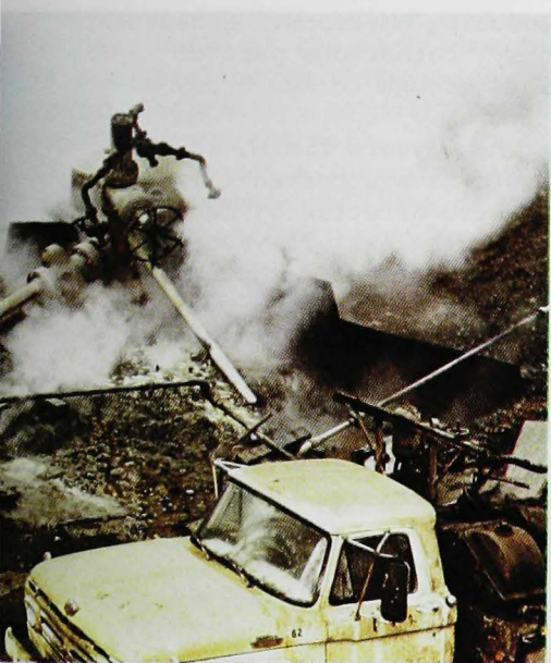
Figure 5. Steam well blowout at the Geysers Field, California. Illustrates the need for precautions to prevent blowouts from occurring even at producing fields.
