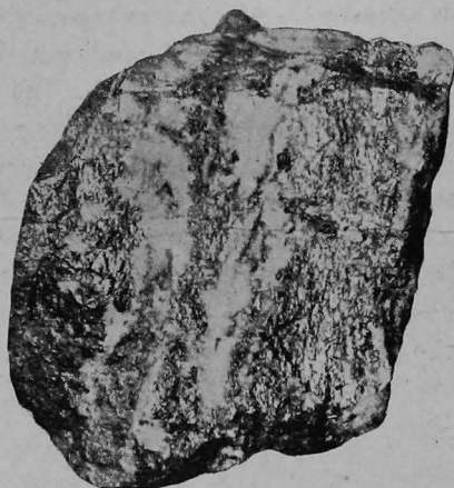
Fig. 26. Ore from the Fidelity mine. The white mineral is quartz and the gray is pyrite. Note the banding. This specimen is characteristic of the pay streak of this vein.
