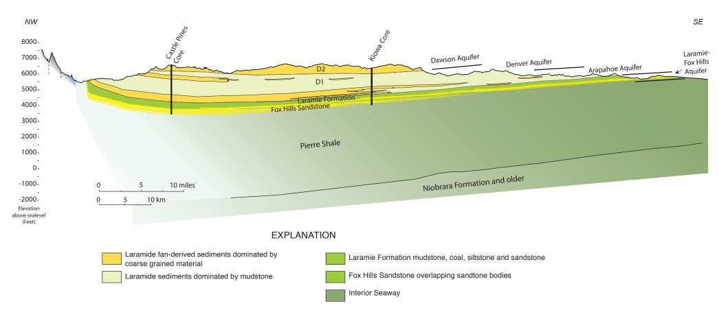
Figure 11b-02-01-03. Denver Basin cross section showing different geologic units and aquifers. Colorado Geological Survey ON-010 Colorado Groundwater Atlas.
