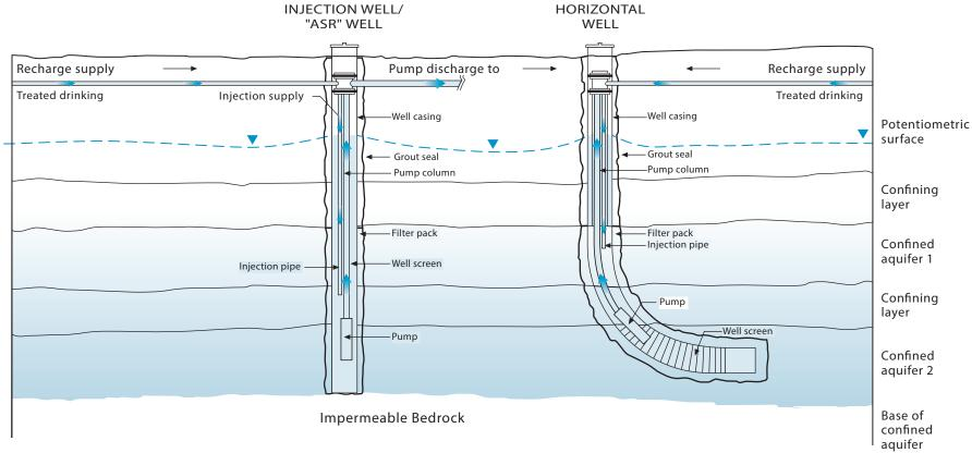
Note: Alternatively, the pump column, equiped with a down-hole flow control valve, can serve as the injection pipe.
